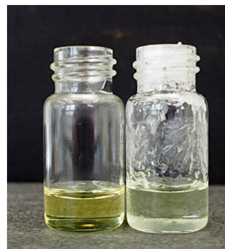
Fig.12. Hydranal-Coulomat AG (left) and Reagent M (right) after four days in open vials.
